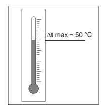
During the running in period (first 200-300 hours), the temperature increase t may be even 25% higher. In mounting positions V1-V5 (vertical position with the output shaft facing downwards), the temperature values may be even 10% higher than those measured in the B3/1U position. This is because of the increased amount of oil inside and the different way in which the coolant splashes around.
